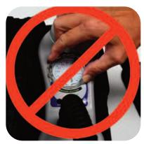
**ATTENTION:** Never turn the dial when the device is under pressure as this will immediately cause the instrument to break.
