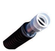
Take adapter number #1 and firmly push it into the grey tube in the end of the hose. Make sure that the adapter is fully seated on the tube by pushing it until the end of the tube pushes past the raised ring in the adapter.
