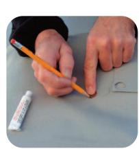
Wait about 5 minutes or until the surface of the glue hazes over then apply the patch. Do not apply wet glue to wet glue.
