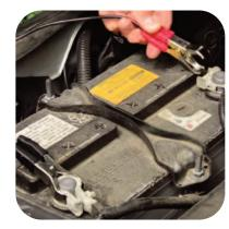
WARNING: Always connect red clip to the positive pole and the black clip to the negative pole. Cross connecting wires could damage both the pump and boat.
