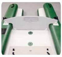
Motor Mount Transom Board Insert motor mount transom board into motor mount grommets with small plate facing forward.
