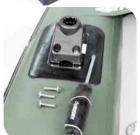
Attach deck mounts with 7/8" screws provided to the pad mounts at the bow & near the transom. Screws are located in Orange Repair Kit.
