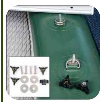
Near valves in bow (front) are four D-rings (two on each side of boat) that hold the aluminum board to the boat.
