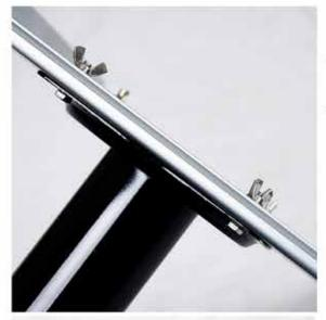
Attach swivel seat to the aluminum board using 1" hex head bolts and wingnuts.
