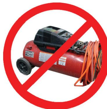
**Warning:** Air compressors that are designed for other uses, like tire inflation (usually around 32 PSI) can easily harm your Sea Eagle which works at a much lower pressure. For this reason we recommend only using Sea Eagle pumps.
