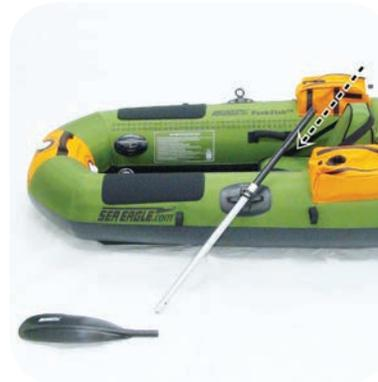
Push the drip guard onto the shaft all the way to the black grip. Insert shaft in oarlock ring.
