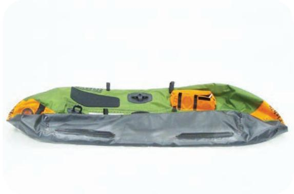
Fold one side over the floor. The bottom should be exposed 2-3 inches past the tracking strips.
