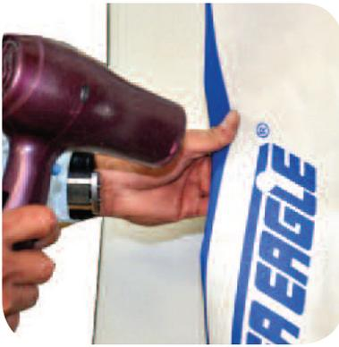
Use a hair dryer on the high setting to activate the adhesive and then press firmly on the patch until it cools.
