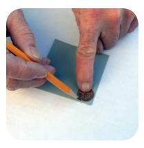
Trace the outline of a penny on the patch material and cut using scissors. Trace the outline of the penny on the boat. Coat the patch and boat with the repair kit glue.
