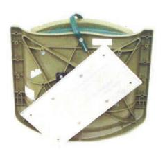
Attach front and rear crossbars to the aluminum seat board. Run bolts up through the bars and through the plate. Place washer over the bolt on top of the plate. Tighten knob after second bolt is inserted.
