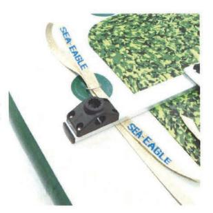
Move the loop so it can go around the bar and rod holder base.
