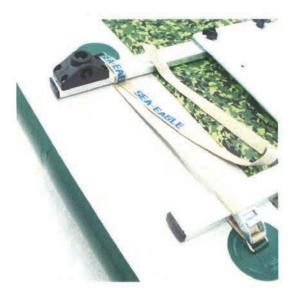
Pull the strap tight and run the free end through the buckle.
