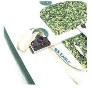
Slide the strap under the bar and over the rod holder base.
